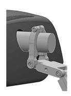
4 - Most compatible mirrors have a stem between the mirror and the windshield that has a pivot on both ends. We recommend that you try moving the mirror upward before installing the mount. Grab the mirror and move the stem upward using the windshield pivot only. Adjust the mirror to your normal viewing position using the mirror pivot only. Notice the higher location of the mirror as shown above. NOTE: The mirror stem may move side to side as well.
