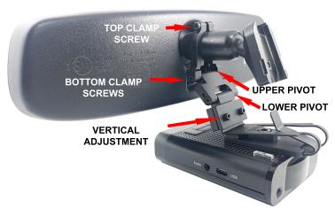
6 - Install the RD onto the mount. Make the necessary adjustments as shown above. Using the upper and lower pivots, and the vertical adjustment, leave enough room below bottom of mirror to allow access to buttons on top of radar detector.
